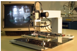
The BGA936ES builds every type of BGA & SMD, only needs to change the NOZZLE.
