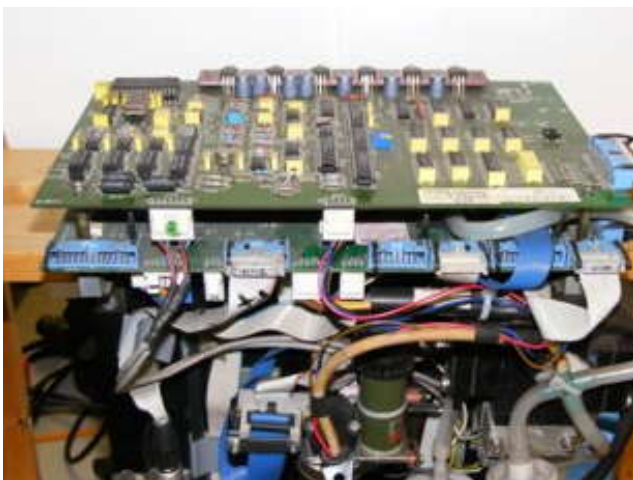
Complete Head Assembly including Bearings, Fiducial camera, Z-Axis boards etc.
