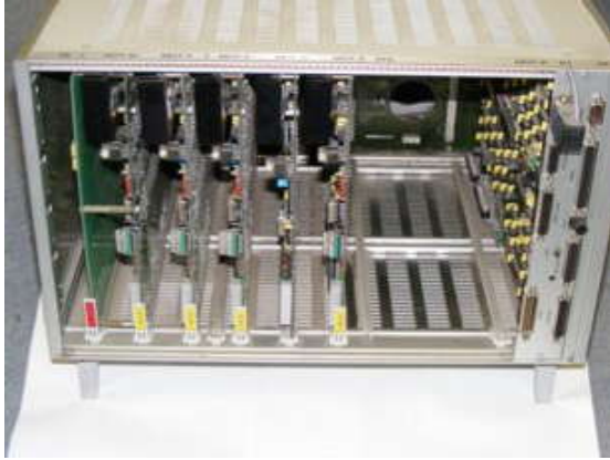
Complete Card Rack including Motor controllers, Vision Card and Feeder Control cards.
